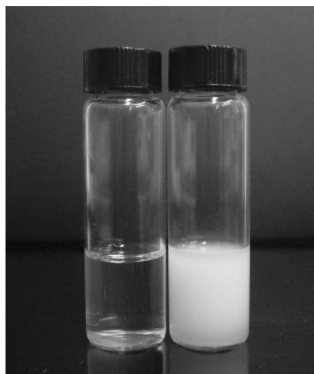
Fig. 4 Temperature-induced reversible micellization behavior of Den 30 in water at 25 \text{ }^\circ\text{C} (left) and at 75 \text{ }^\circ\text{C} (right). The concentration is 2.7 \text{ g L}^{-1} .
